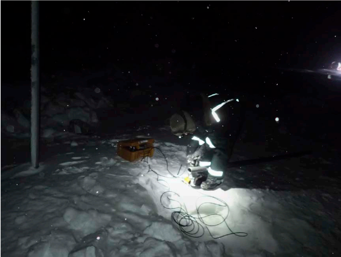
Fig. 2. The ADCP site marked with a pole. We are making the camera ready to be lowered. Note the front of the pressure ridge in the background.
